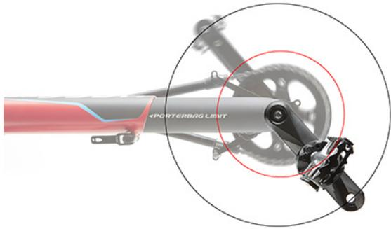
The new Crank Shortener has a wider adjustment range. Four small screws provide more comfort and safety.
