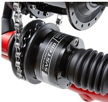
Easier shifting on steep climbs: a new differential sans freewheel is now available for all trikes with hub gears.
