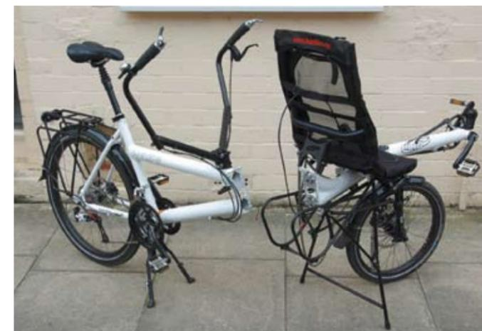
The frame itself is neatly TIG-welded in aluminium, with a thick, good quality powder coat finish. Front and rear halves each house a substantial headset – one for the forks, the other for the handlebars. Between the two is the frame joint, a
