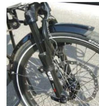
**A 203 mm disk plus suspension forks offer control and comfort for the heavily loaded front wheel.**
