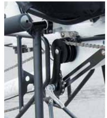
Below the frame, the linkage to the front wheel is solidly made, with a big shiny elastomer fitted to the push-rod to prevent any damage where it hits the frame and, I assume, to provide a nice soft limit to steering lock.
