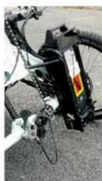
ABOVE: The battery is neatly mounted low down on one side.
