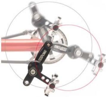
The crank for a smaller pedal rotation – e.g. for riders with limited knee flexibility.
