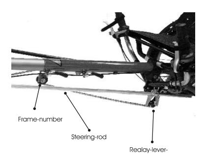
By pressing the relay lever clip together, the steering rod can be pushed into the required position.
