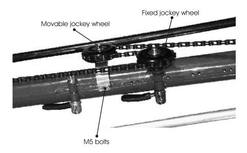
If further adjustment is necessary, the movable jockey wheel must be removed by unscrewing the M5 bolts. The trike length should be adapted as described above and the jockey wheel secured in a suitable hole position.
